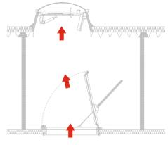
Example of installation in internal suspend sealing with housing for smoke and gas ventilation
