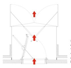
Schematic diagram of "roof hood" with NRWG and cool it hatch
